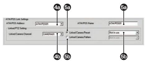
Figure 109. Event-PTZ Link Settings: Linking Presets and Patterns to ATM/POS Events
